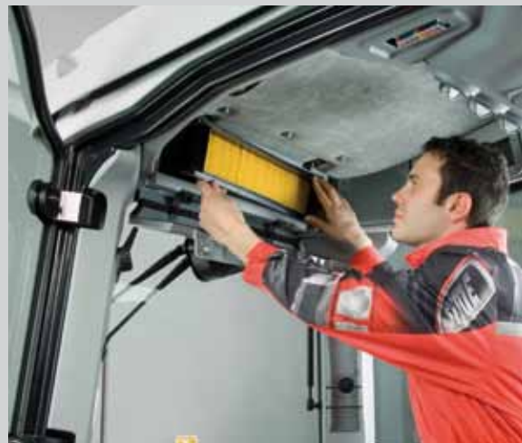
The internal cab air filter is easy to access without tools.
