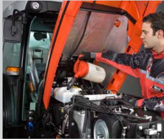
Topping up the coolant is safe and simple.
