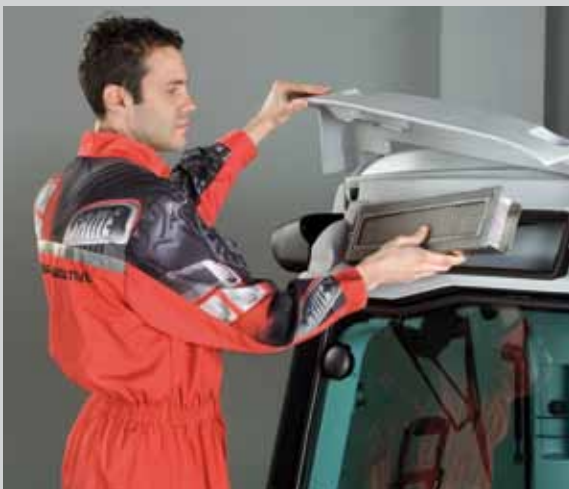
The external cab air filter is easy to access without tools.
