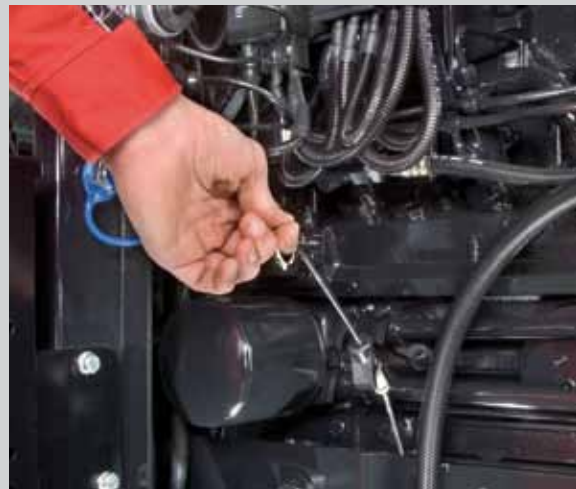
You can check the oil level without lifting the hood or removing the side panels.
