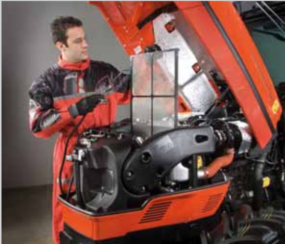
For maximum ease of maintenance, the radiators are equipped with a fly-screen that traps dust and other particles.
